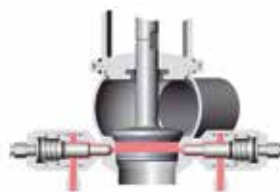
Valve closed. Leakage valves open for draining or cleaning of the leakage chamber.
