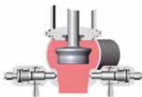
Valve open. Leakage valves closed.
